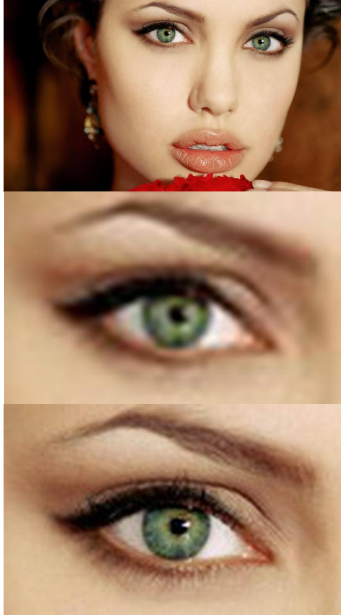
Fig.33 Image interpolation using linear method of interp2 built-in MATLAB® function. Top: original image. Medium: close-up of eye in image. Down: interpolated image.
