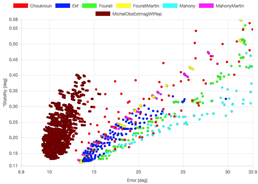
Figure 16: Spectrum of possibilities in terms of stability/precision in AR with high magnetic perturbations
