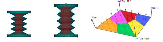
**Figure 3.** Pneumatic actuation of a soft body with a cavity, at rest (left) and with the cavity inflated by air pressure (middle). The pressure applied on the cavity walls is integrated using the surface of triangles and distributed on the vertices (right).
