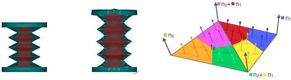
**Figure 3.** Pneumatic actuation of a soft body with a cavity, at rest (left) and with the cavity inflated by air pressure (middle). The pressure applied on the cavity walls is integrated using the surface of triangles and distributed on the vertices (right).
