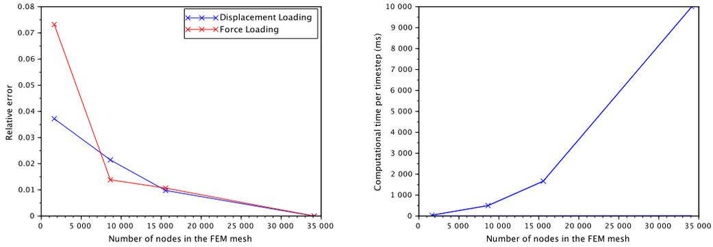
**Figure 8.** Relative error (left) and computation time (right) of Diamond robot simulation when varying the refinement of the mesh. The relative error is computed for the end-effector position when actuating three of the four cables.
