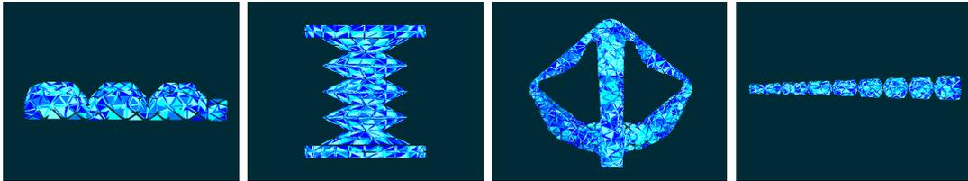
**Figure 1.** Three dimensional volume mesh of some of the robots presented in the paper. From left to right: one soft finger actuated by one cable (see Flexo 7.2.2), one pneumatic element of Fetch 7.2.1, a parallel like soft robot (Diamond 7.2.3) and a soft trunk actuated by 8 tendons (see 7.2.5).
