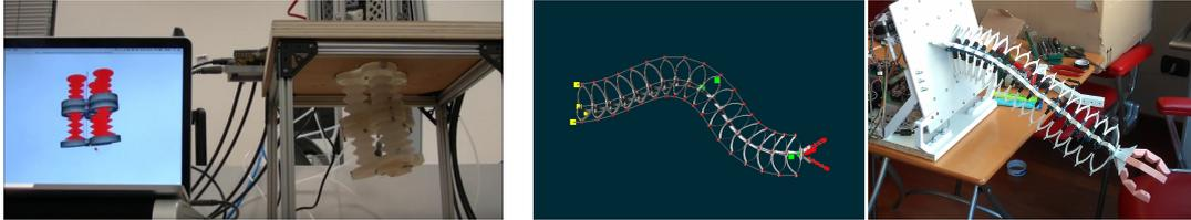
(a) Control from inverse simulation of two Fetch platforms stacked for the Soft Robotic Toolkit 2015 competition. (b) Simulation of Flexo (left) and the real robot (right).
