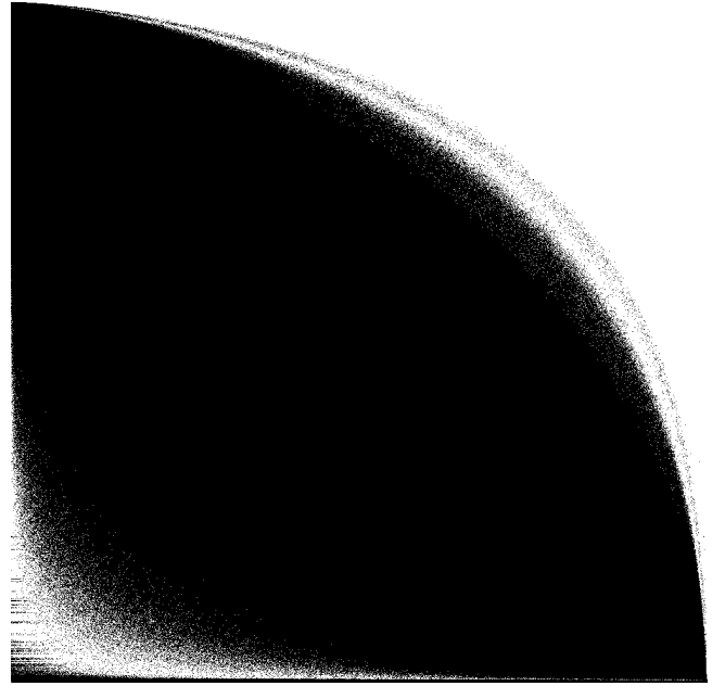
Figure 3: Pattern of the GL7d19 matrix. The Faugère-Lachartre heuristic finds much more pivots after a horizontal flip.
