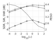
Fig. 1: The performance measures as a function of  $\delta$  for CTF-MINT (*left*) and  $\kappa$  for CTF-MPDR (*right*). I=4 and J=3. The input SNR is 10 dB. SDR, SIR and PESQ of the unprocessed signals are -6.9 dB, -3.0 dB and 1.85, respectively. Two vertical axes are used due to the different scales and units of the performance measures.
