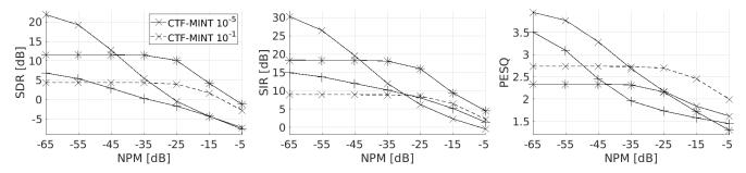
Fig. 5: The performance measures as a function of NPM, I = 4 and J = 3. The microphone signals are noise free. SDR, SIR and PESQ of the unprocessed signals are -6.9 dB, -3.0 dB and 1.85, respectively.
