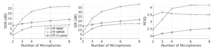
Fig. 2: The performance measures as a function of the number of microphones, J=3. The microphone signals are noise free. SDR, SIR and PESQ of the unprocessed signals are -6.9 dB, -3.0 dB and 1.85, respectively. Note that the legends in this figure are common to all the following figures.
