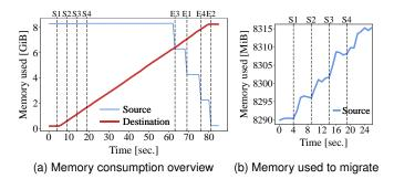
Fig. 4. Overview of the memory consumption on both source and destination servers during 4 parallel migrations. Figure (b) is a closest view of the source server consumption when the migrations begin.
