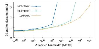
Fig. 3. Duration of a live-migration between 2 KVM hypervisors depending on the allocated bandwidth and the parameters used by the command *stress* to generate dirty pages. *1000\*10K* indicates the VM runs 1000 concurrent threads that continuously allocate and release 10 KiB of memory each. The VM memory used is set to 4 GiB and the downtime is limited to 30 ms.
