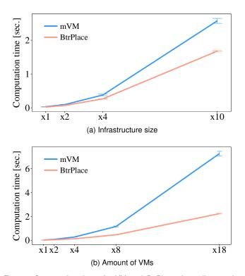
Fig. 12. Computation time of mVM and BtrPlace depending on the scaling factor
