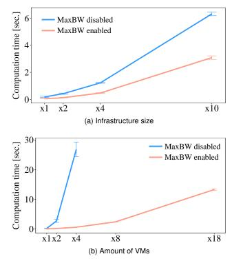
Fig. 11. Comparison of the mVM solving duration depending on the *MaxBandwidth* optimization and the scaling factor. When the *MaxBandwidth* optimization is disabled, each migration has 4 different bandwidth allocations allowed by steps of 250 Mbit/s.
