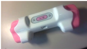
Fig. 2. Upper-limb-grasp motion measurement Controller (System Instruments Co.,Ltd.)
