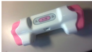
Fig. 2. Upper-limb-grasp motion measurement Controller (System Instruments Co.,Ltd.)
