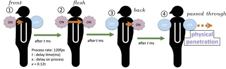
Fig. 5. Vibration-motor controls with delay for physical penetration
