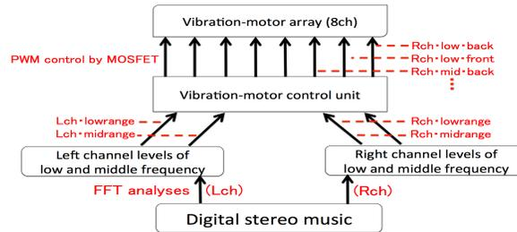
Fig. 1. System structure
