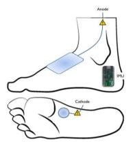
Figure 1 Electrodes and IMU locations. To deliver the stimulation, a self-adhesive electrode is placed as the cathode on the arch of the foot and a common anode is placed on the dorsum of the foot.
