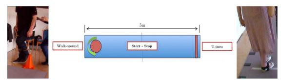
Figure 4 Five meters experimentation path. The subject starts in the middle of the walkway, walks 2,5 m, performs a u-turn at the line, goes back 5 m, walks around a cone, walks back 2,5 m then stops where he started.
