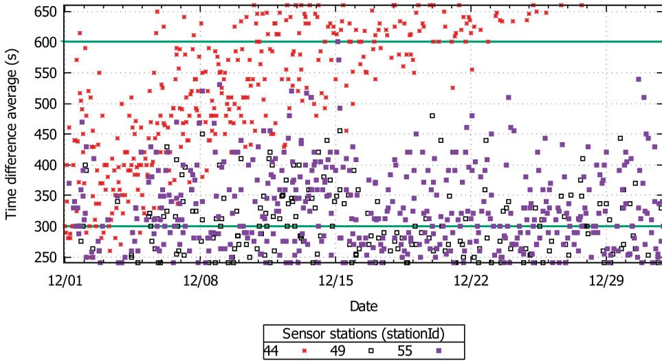
**Figure 8.** Malfunction sensor station detection during December 2016.
