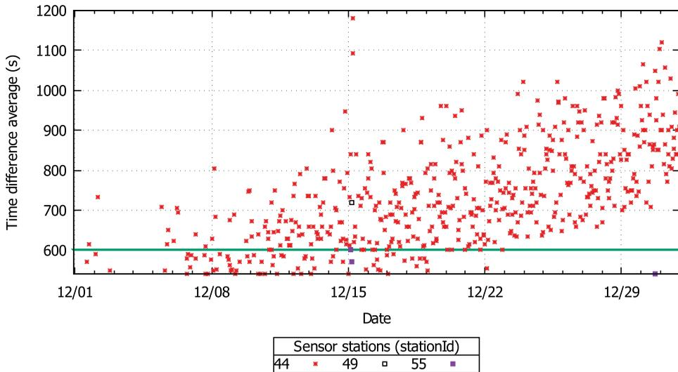
**Figure 9.** Failure sensor station detection during December 2016.
