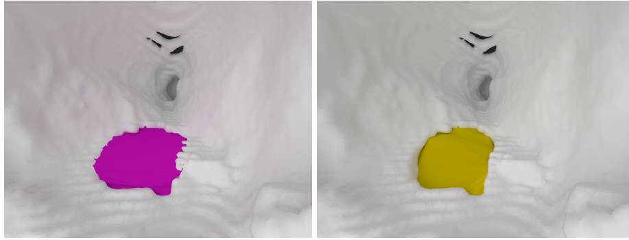
Fig. 6. 3D visualization of fracture extraction : manual point selection (pink), automatic point selection (yellow)
