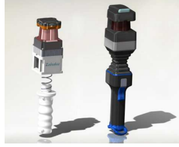
Fig. 6. Zebedee design of 3D LRF with 2D LRF mounted on spring [1]
