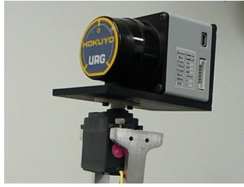
Fig. 5. First known design of 3D LRF with servo [10]
