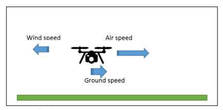
Fig. 6. Analysis od UAV speed in windy environment (up wind flight)
