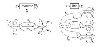
Fig. 5. Component models monitor (left) and line (right)
