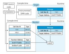
Control Flow Integrity (CFI): shadow call stack
