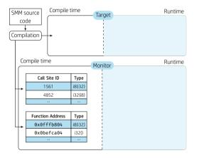
Control Flow Integrity (CFI): type-based verification We focus on indirect branches integrity
