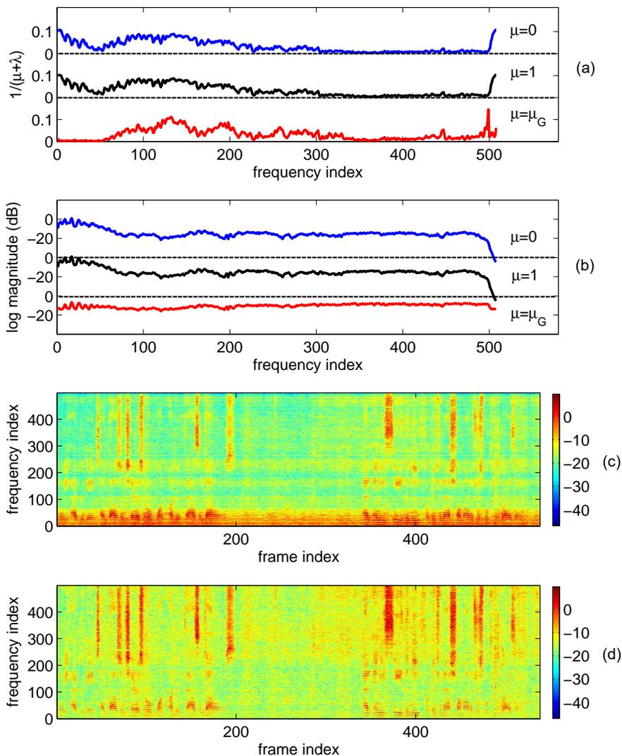
Figure 3: Illustration of the r1MWF- $\mu$  filter for an example sentence (M06\_440C0201\_BUS) from the real test set. (a) Spectral gain along frequency for different values of  $\mu$ . (b) The corresponding log-magnitude of one frame of the filtered signals. (c) and (d) Log-magnitude spectrograms of the filtered signals with  $\mu = 1$  and  $\mu = \mu_G$ , respectively.
