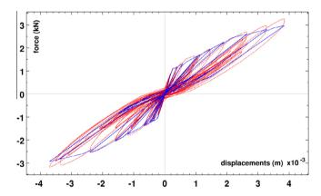
**Fig. 6-2.** SAFE shear-wall experimental program: wall T5; comparison between test (dotted red line) and model (continuous blue line) results. (For interpretation of the references to colour in this figure caption, the reader is referred to the web version of this article.)
