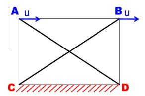
Fig. 6-1. Equivalent RC connecting rods representing SAFE RC wall T5.
