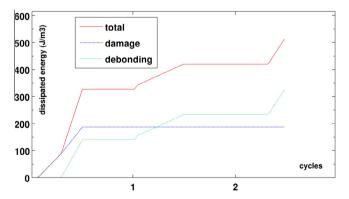
**Fig. 5-4.** Damage (blue), debonding (green) and total (red) dissipated energy over time for a symmetric alternate loading on two strain-controlled cycles. (For interpretation of the references to colour in this figure caption, the reader is referred to the web version of this article.)
