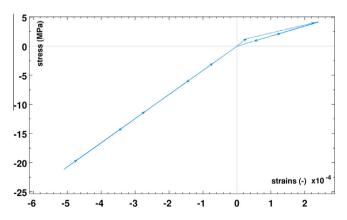
Fig. 4-1. Stress-strain cyclic response of concrete damaged through the damage
