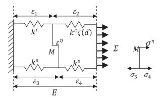
$\textbf{Fig. 3-2.} \ \ \textbf{Rheological model representing schematically the unit cell of Fig. 2-2 in one dimension.}$
