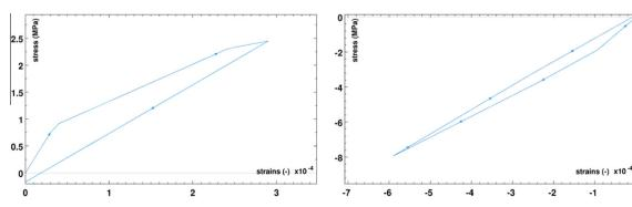
Fig. 5-1. Typical behaviour in tension (left) and compression (right) for damage-debonding model.
