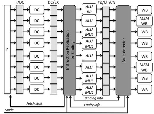
Fig. 2: Hardware components inserted in the VLIW pipeline.
