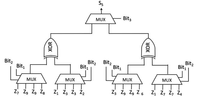
Fig. 8. Proposed stochastic implementation of edge detection algorithm
