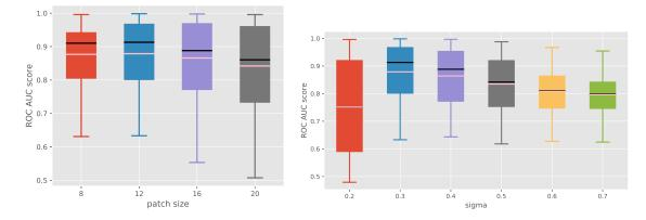
Figure 8: The impact of the choice of hyper-parameters on prediction performance in *top* mode: influence of patch size l while fixing  $\sigma = 0.3$  (left) and influence of kernel parameter  $\sigma$  while fixing patch size l = 12 (right)
