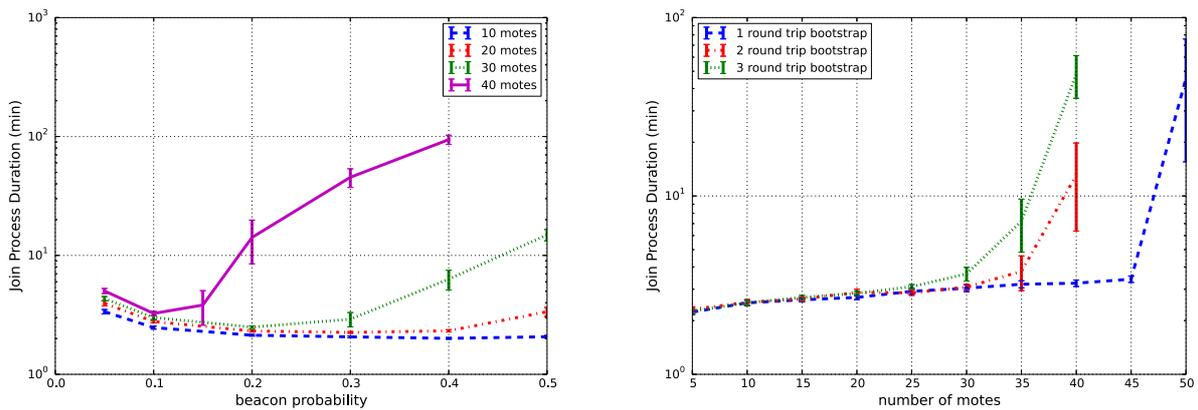
**FIGURE 2** a) Join duration for a single round trip bootstrap protocol and  $p_{DIO} = 1/3$ . For smaller values of  $p_{EB}$ , the dominant component of the duration is the time the mote spends unsynchronized waiting for EBs. For larger values (and increased traffic load) bootstrap retransmissions prevail. b) Join duration for beacon probability  $p_{EB} = 0.1$  and  $p_{DIO} = 1/3$ . For a given join process duration, the number of motes in the network decreases with increasing traffic load.
