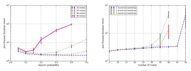
**FIGURE 2** a) Join duration for a single round trip bootstrap protocol and  $p_{DIO} = 1/3$ . For smaller values of  $p_{EB}$ , the dominant component of the duration is the time the mote spends unsynchronized waiting for EBs. For larger values (and increased traffic load) bootstrap retransmissions prevail. b) Join duration for beacon probability  $p_{EB} = 0.1$  and  $p_{DIO} = 1/3$ . For a given join process duration, the number of motes in the network decreases with increasing traffic load.
