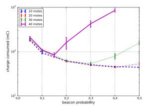
**FIGURE 3** Charge consumed during the network formation assuming a LTC5800 System-on-Chip is used. The value of  $p_{EB}$  that minimizes energy consumption is slightly higher compared to Fig. 2 a due to the initial unsynchronized period where motes constantly listen for EBs.
