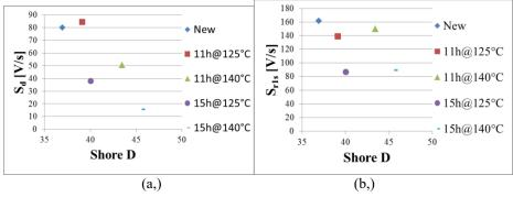
**Fig. 5.** Slope of decay voltage  $(S_d)$  versus Shore D hardness (a,) Slope of return voltage after 1 s shorting time (Sr1) versus Shore D hardness (b,)
