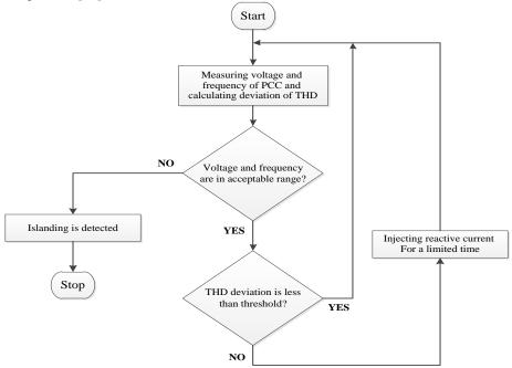
Fig. 2. Islanding detection by suggested method
