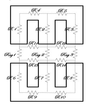
Fig. 3. Simplified equivalent magnetic circuit.
