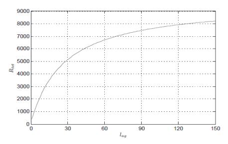
Fig. 5. Variation of total magnetic reluctance function of the air gap.
