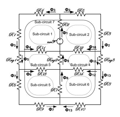
Fig. 4. Equivalent magnetic circuit with sub-circuits.
