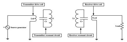
Fig.1. Simplified equivalent circuit of the WPT system.
