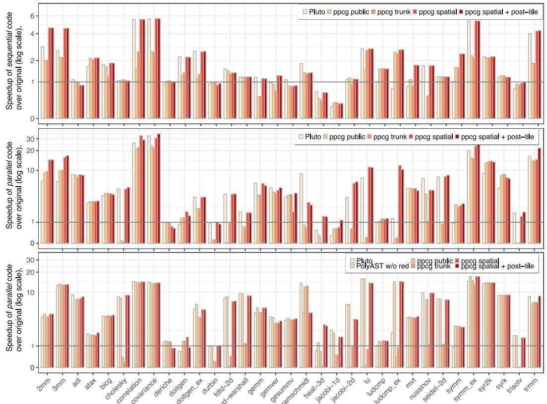
Figure 3: Speedup of the optimized tiled code over the original code with different scheduling algorithms; top: sequential code on **skylake**, middle: parallel code on **ivy**; bottom: parallel code on **westmere**.
