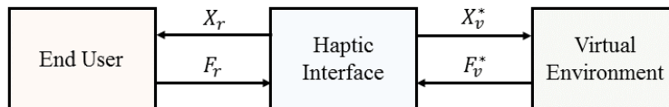
Fig. 1. An overview of the interaction between the user, the HI and the VE.
