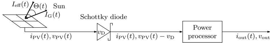
Figure 3: Using a fraction  $I_{\text{eff}}$  of the solar irradiance  $I_G$ , the PV cells generate a power (current  $i_{\text{PV}}$  and voltage  $v_{\text{PV}}$ ) that goes through a Schottky diode and a power processor before it can be consumed
