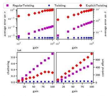
Fig. 4: Evolution of the performance of the controllers with respect to the gain.
