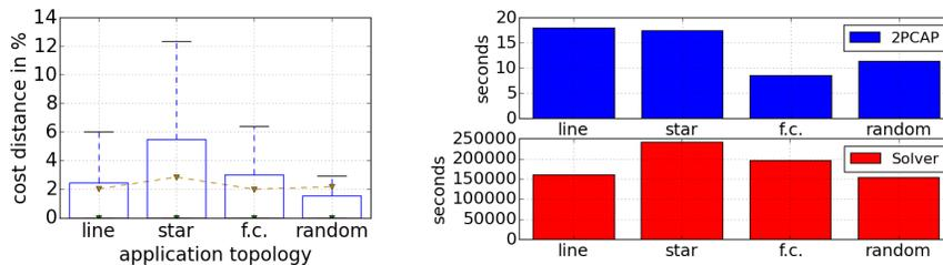
**Fig. 3.** (Left) Cost distances as percentage of 2PCAP solutions compared to optimal solutions aggregated by application topology type. The green solid line is the median and the brown dashed line is the average. (Right) Sum of execution times in seconds from 2PCAP and SCIP solver aggregated by application topology – SCIP: average 4180s, median 1800s. 2PCAP: average 0.1s, median: 0.08s.
