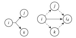
Figure 3: Transformation of a task with a single shared output data into SIMPLEDATAFLOWMODEL. The plain edge carries the shared data size, while dashed edges have null size.
