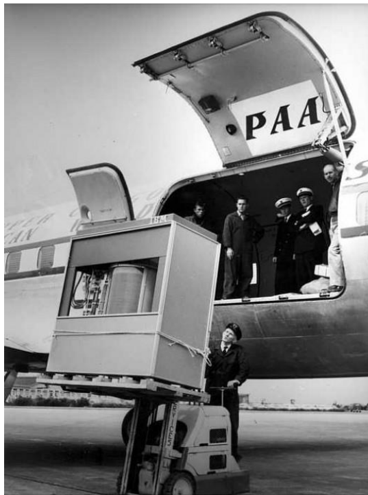
Fig. 1. Flying the RAMAC 305: An IBM 305 disk unit, weighing a bit over a ton, being forklifted onto a Pan American Airways operated Douglas freighter aircraft (most possibly a DC-6A), ca. 1956
