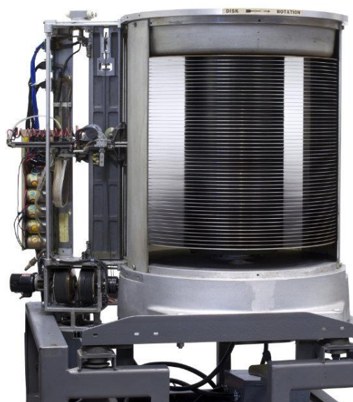
Fig. 3. IBM Corporation, RAMAC actuator and disk stack, 1956. 54in x 40in x 30 in. “This is the heart of the world’s first disk drive. It has 50 24” disks spinning at 1,200 RPM holding 5 million characters of information.” Photo: Mark Richards. (Source: Computer History Museum, Mountain View, CA. Object ID: L2009.1.1p.)
