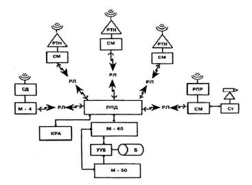
**Fig. 4.** Computer network of an experimental missile defense system 1955/56. Source: V. S. Burtsev, Distributed Systems: The Origins of Computer Networks in the USSR, in: G. Trogemann et al. (eds), Computing in Russia. Braunschweig 2001, pp. 215-220.
