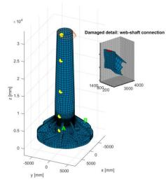
Fig. 1 MB foundation for a mobile met. mast at Horns Rev 2 (2009) (left). FE-model of the MB for numerical simulations (right). Bi-axial x-y accelerometers are illustrated by yellow dots.
