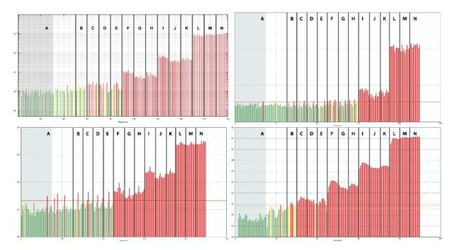
Fig. 2 MD-based damage indicators (upper left). Classic subspace-based damage indicators (upper right). Robust subspace-based damage indicators (lower left). Fusion of the subspace-based and MD-based damage indicators in the Hoteling control chart (lower right).
