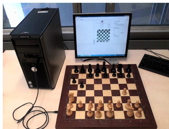
Figure 1. DGT electronic chessboard connected via USB to a computer.
