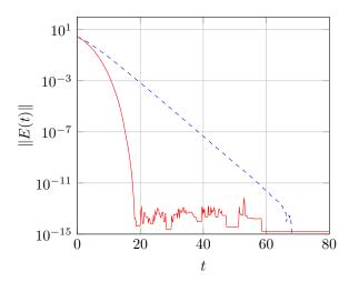
Fig. 3. Comparison of the error for the linear (dashed) and finite-time (solid) observer
