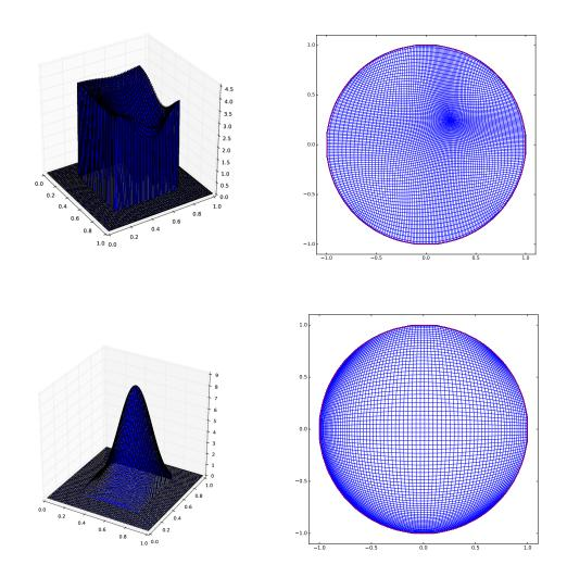
Figure 6: Left column: Source density f. Right column: Corresponding optimal map deformation of the grid.
