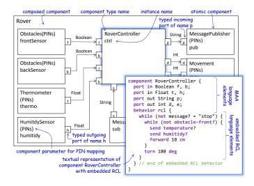
Fig. 7. Example RASPIROVER DSL model defined in MONTICORE
