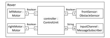
Fig. 1. Example rover hardware architecture defined with RASPIROVER DSL
