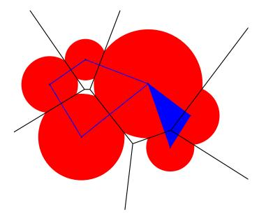
Figure 6.2: Union of balls and  $\alpha$ -shapes.
