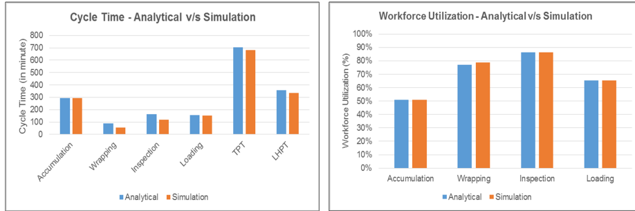
(a) DC Cycle Time Comparison: Analytical v/s Simulation (b) DC Workforce Utilization Comparison: Analytical v/s Simulation
