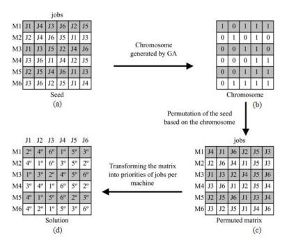
Fig. 2. Representation schema of FT06 instance
