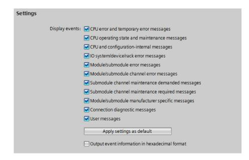
Figure 10. Engineer-defined events recorded by the diagnostics buffer.
