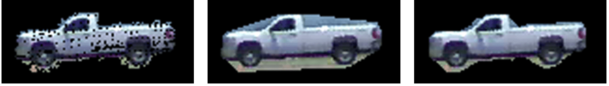
(a) Estimated vehicle template using DBSCAN, with holes due to errors in hull of the cluster in (a). Note this is with the alpha complex. (b) Vehicle template using the convex hull. (c) Estimated template computed DBSCAN, with holes due to errors in hull of the cluster in (a). Note this is with the alpha complex. (d) an intermediate result.
