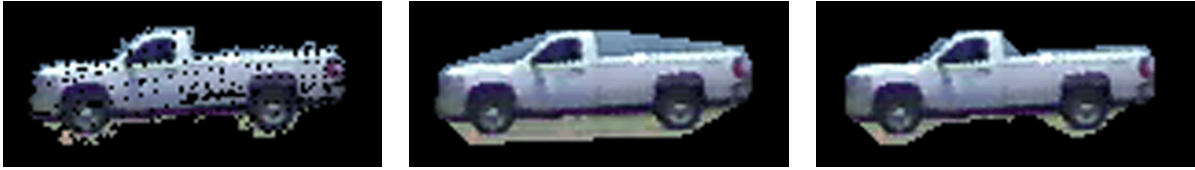
(a) Estimated vehicle template using DBSCAN, with holes due to errors in hull of the cluster in (a). Note this is with the alpha complex. (b) Vehicle template using the convex hull. (c) Estimated template computed with the alpha complex.
