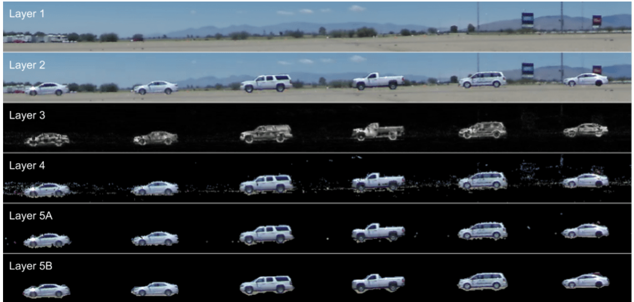
Figure 2: Step-by-step visualization of background subtraction methods. Layer 1 shows a section of the estimated background within the first 15-second time interval in Experiment A. Layer 2 is the first frame of that time interval. Layer 3 is the square distance between layer 1 and layer 2. Layer 4 is the remaining foreground after removing pixels at locations that have square distance under 14. Layer 5A is the refined foreground after applying morphological transformation on layer 4. Layer 5B is the refined foreground after removing noise pixels outside the alpha complex of every vehicle from layer 4.
