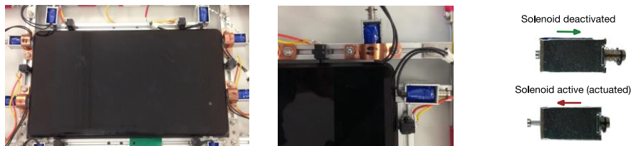
Fig. 1. Picture of prototype device. The device captures 2D touch location and 2D shear input. Each solenoid on the side of the tablet can be activated independently to lock a specific axis of the shear input (e.g., based on the touch input of the user).
