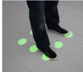
**Fig. 10.** Alternative floor display using a ceiling-mounted short-throw projector.
