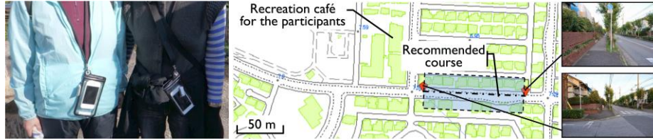
Fig. 4. Left: User wearing the device. The device is slung around the user's neck and fitted inside the user's jacket. Right: A brief overview of the recommended walking course.
