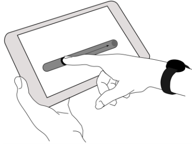
Fig. 1. SwipeID. Associating touch data with IMU data using a challenge-response protocol.
