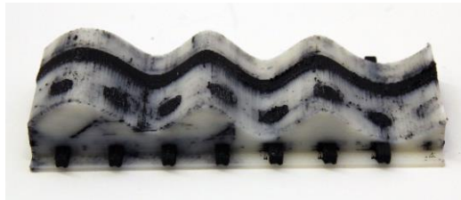
Fig. 2. Slider printed onto a decaying sine wave
